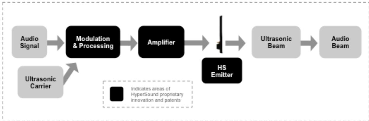
**Figure 3: Diagram of HyperSound Process:** Figure 3 displays a functional diagram of HyperSound’s audio beam system. First, the emitted ultrasonic wave is inaudible, but as it impresses audio signals onto the carrier in the air, the audio signal is demodulated by the parametric array effect and becomes audible. This demodulated audio wave retains the directivity of the ultrasonic wave, thus producing an audio beam.
